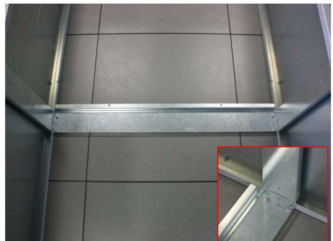
Fig. 4: traversa mediana / middle horizontal panel
